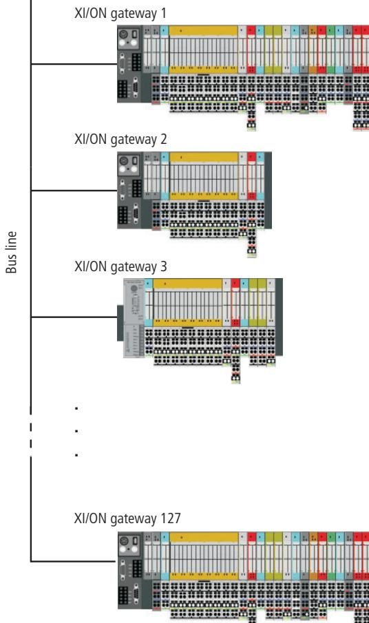
Figure 31: Max. system configuration of a CANopen bus line
