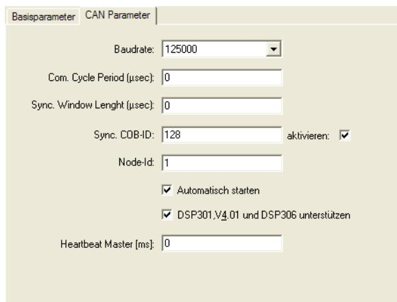
Figure 34: CAN parameters of the CAN master
