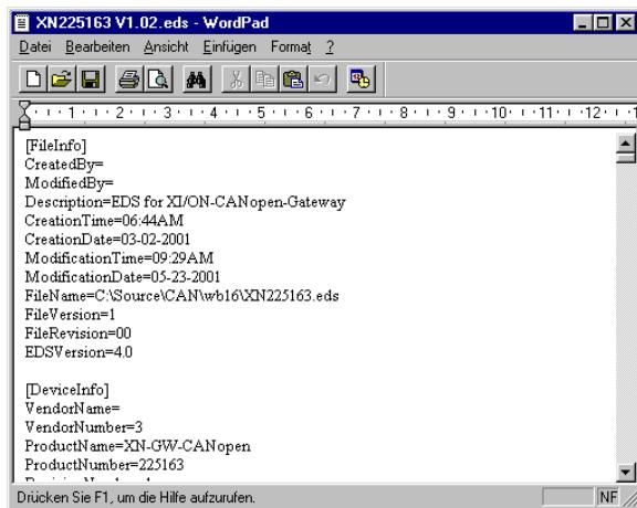
Figure 29: Header of an EDS file for XI/ON
