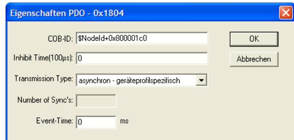
Figure 39: PDO properties (Send PDO mapping)
