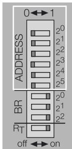
Figure 25: DIP-switches on the gateway
