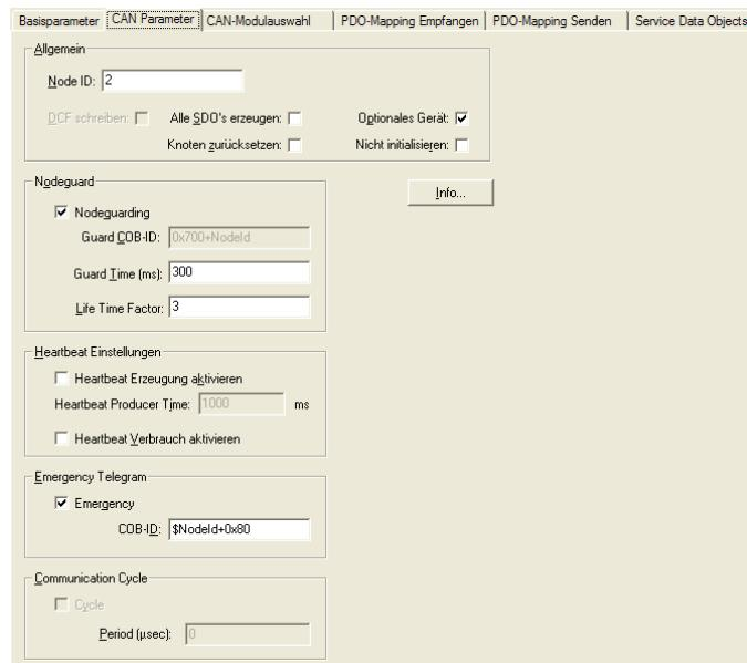
Figure 36: CAN parameters of the CAN slave (in this case: XN-GWBR-CANopen)
