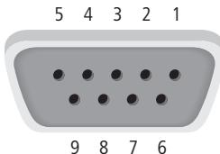
Figure 5: SUB-D socket on the gateway (top view)
