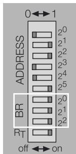
Figure 27: DIP switches for setting the bit rate
